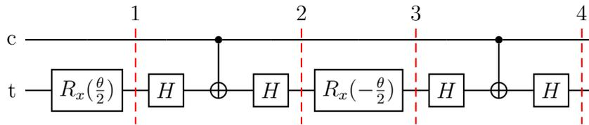
Figure 1: Circuit for controlled rotations around  $x - axis$
